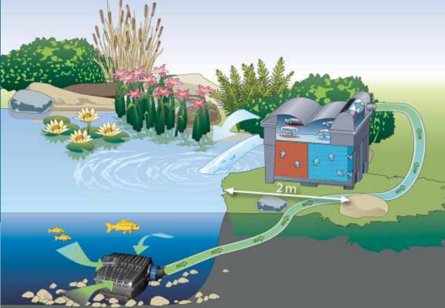
Schematic diagram: Filter and watercourse pump AquaMax Eco Classic (START) in combination with an OASE flow-through filter, BioSmart (START)
